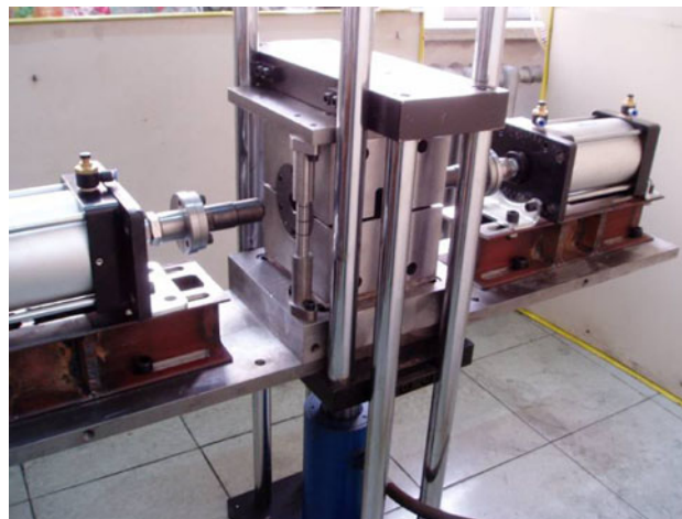
Fig. 2 Experimental set-up for tube bulging test
